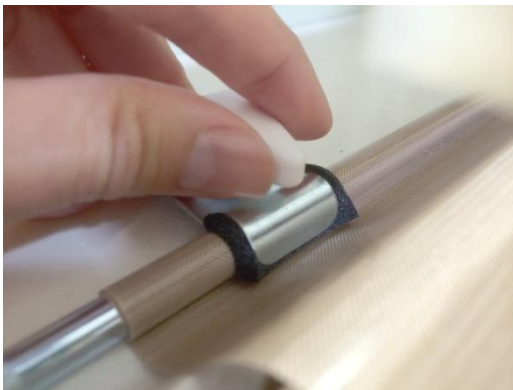
Figure 7. Loosen multi-star knob to remove the PTFE roller.
